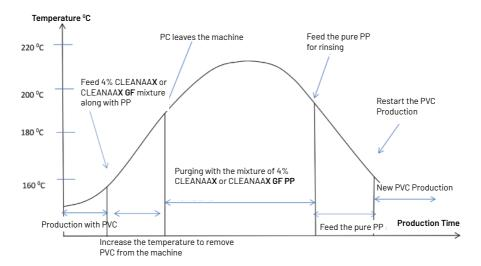
When purging a machine using PVC in production, we recommend using "PP" polypropylene as a carrier polymer in the purging mixture. Using "PP" as a carrier polymer during the purging process enables you to reach the temperature range of 200–220°C. Therefore, "PP" is quite stable at this temperature. When rinsing is done with pure "PP", the temperature will be reduced to 165–185°C, and the machine is ready to work with PVC again.
